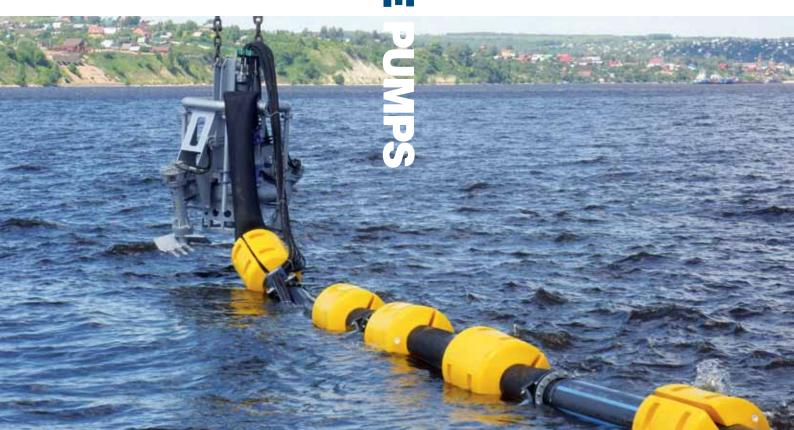
submersible agitator pump technology allows a much higher solid concentration in the dredged slurry thus permitting lower operational cost per cubic meter of material extracted. This means it is possible to reduce discharge line diameter and water usage together with an overall reduction of fuel consumption per extracted ton.
