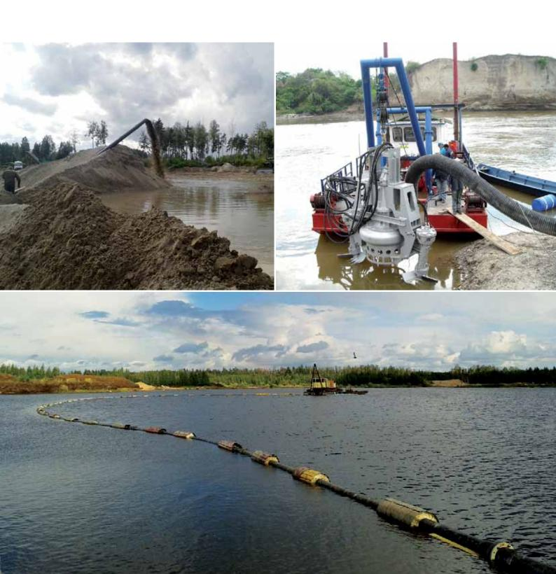
Sand washing and dewatering processes produce a highly abrasive sludge that has to be pumped to settling ponds or treatment plants.
